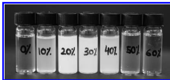
Figure 1. Transparency of TiO 2 /HSEO nanocomposite solutions containing 0, 10, 20, 30, 40, 50, and 60 vol % sol–gel.
